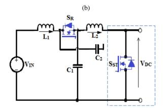
Fig.2.Traditional (a) and its operating (b), synchronous (c) qZS networks
