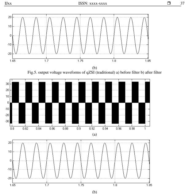
Fig.6. output voltage waveforms of qZSI (synchronous rectification) a) before filter b) after filter.
