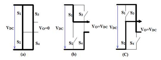
Fig.3. operating states of qZSI shoot through (a), active states (b) and (c)
